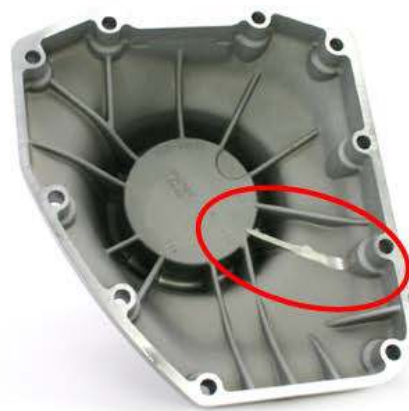
1999-2008, Single Rib Removed
